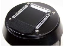
High performance enlarged Pieltier device with side lighting tape-LED in EX-type system.
