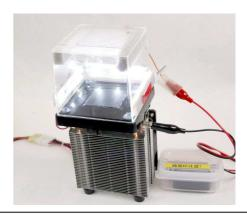
Main unit of standard type (SD) Peltier-cooling cloud chamber.
