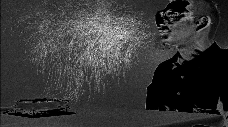
Special video recording was conducted to visualize droplets in the air. Within a range of about 50cm, we can see that droplets emitted by speech from the oral cavity with a "booming" sound are **inhaled and stopped by the filter** in the same way as a mask.
