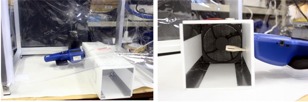
A duct was set up in a clean booth using HEPA filter unit, and the rate at which ultrasonic sprayer mist, simulating droplets from the oral cavity, was captured by a non-woven fabric filter was evaluated. As a result, it was confirmed that **droplets of 5  $\mu\text{m}$  or larger could be almost completely captured.**
