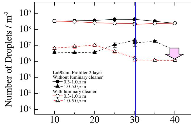
The droplet collection examinations were conducted in a clean bench with a wind speed of about 0.6 m/s. The number of large particles decreased with distance. This may be due to both falling by gravity and shrinking by evaporation.
