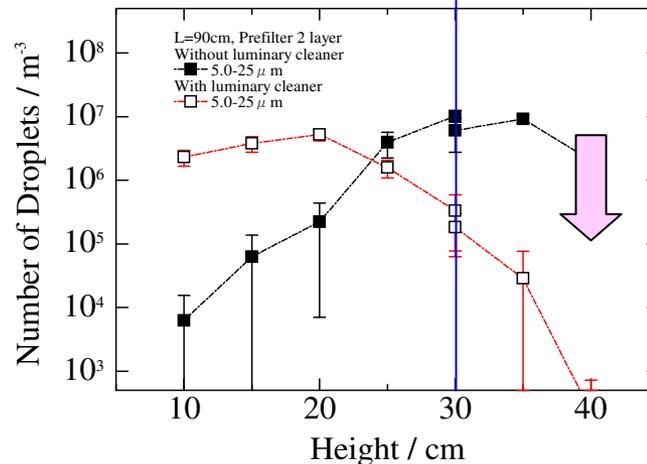
It was confirmed that the **droplet removal system significantly reduced the number of droplets at the level of the face when a person seated at a table.**
